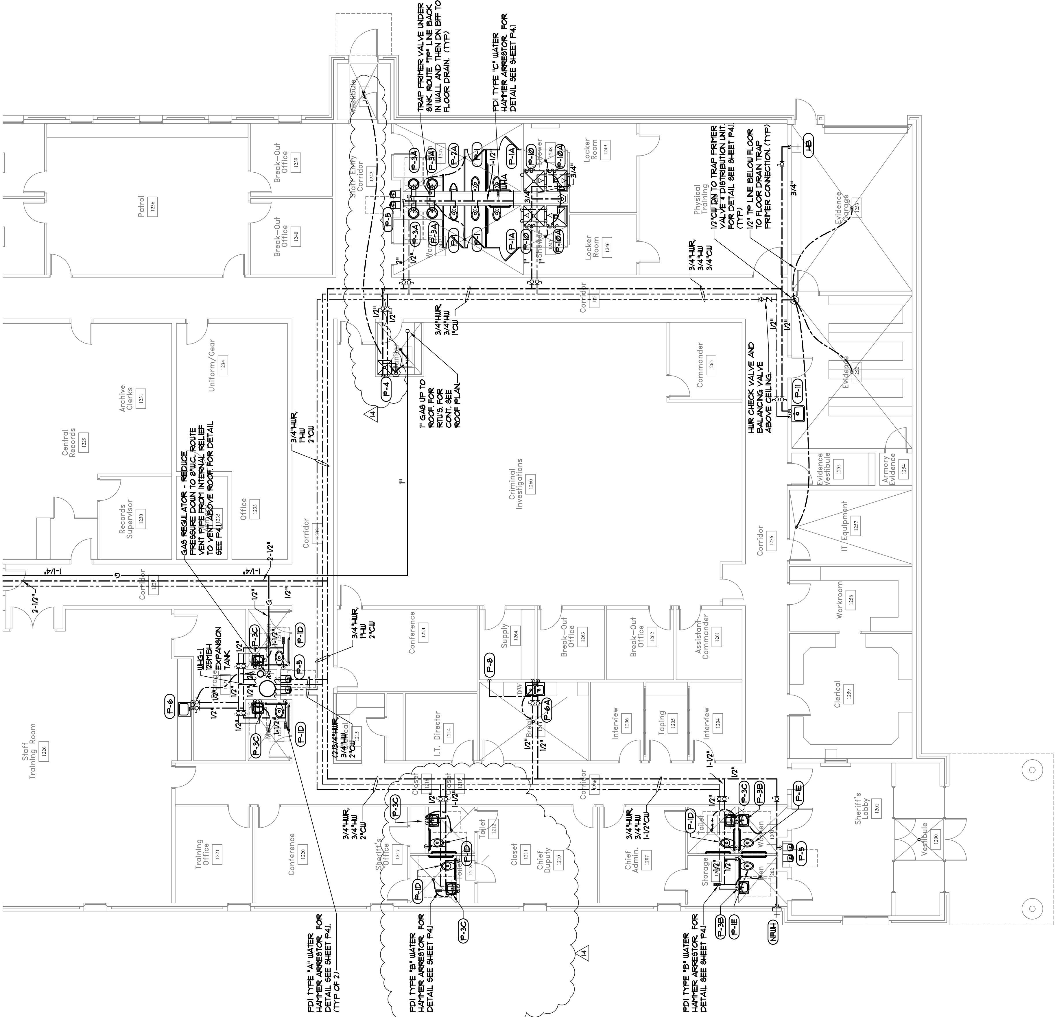
1 PLUMBING PLAN WATER - Area 'A' SCALE 1/8" = 1'-0"
