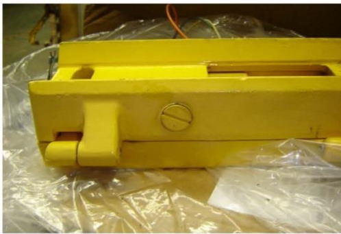
Picture 2 – clamshell mounting bracket with tapped and capped wire entrance hole for wood pole mounting
