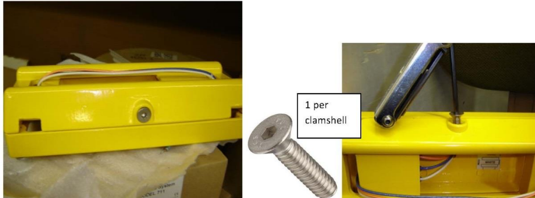
Picture 3 – clamshell mount bracket with flat head 3/16" hex socket closure bolt
