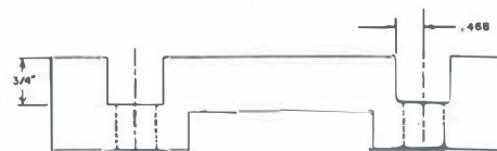
CURB BUMPER MATL: MEDIUM CARBON STEEL
